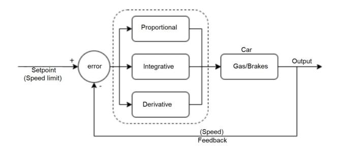
The equation that describes the output for this diagram as a function of time is the following:
