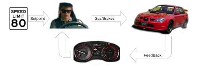
Now that we know what a closed control system is, also called a feedback control system, we can talk about the PID, an acronym for Proportional, Integral, Derivative. This controller will use the current error (Proportional), its integral (Integral) and its derivative (Derivative) to generate an output we will use to act in our system. Its diagram would look like the following:
