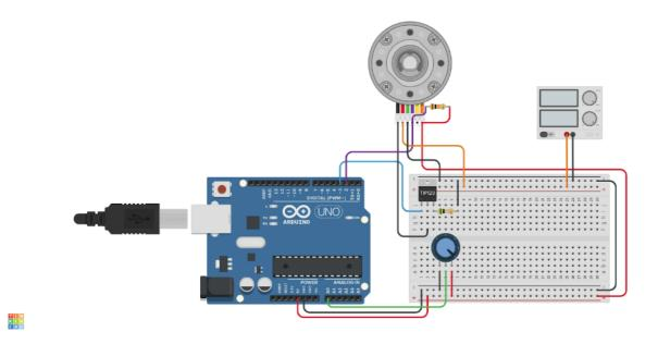
Our circuit consists of a motor we wish to control, with an encoder, a sensor capable of measuring the speed of the motor, and a potentiometer we can use to choose the speed of the motor.
